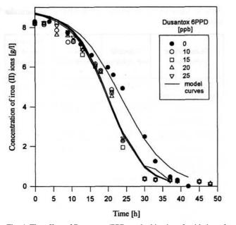
Fig. 4. The effect of Dusantox 6PPD on the kinetics of oxidation of iron (II) ions by *Thiobacillus ferrooxidans* bacteria (Silverman 9K medium,  $37^{\circ}$ C, pH = 2.20).
