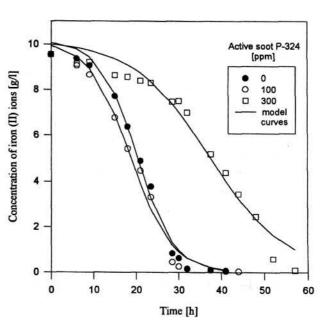
Fig. 2. The effect of active soot P-324 on the kinetics of oxidation of iron (II) ions by *Thiobacillus ferrooxidans* bacteria (Silverman 9K medium,  $37^{\circ}$ C, pH = 2.20).
