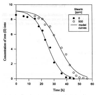
Fig. 3. The effect of stearin on the kinetics of oxidation of iron (II) ions by *Thiobacillus ferrooxidans* bacteria (Silverman 9K medium,  $37^{\circ}$ C, pH = 2.20).
