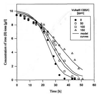
Fig. 6. The effect of Vulkafil CBS/C on the kinetics of oxidation of iron (II) ions by *Thiobacillus ferrooxidans* bacteria (Silverman 9K medium,  $37^{\circ}$ C, pH = 2.20).
