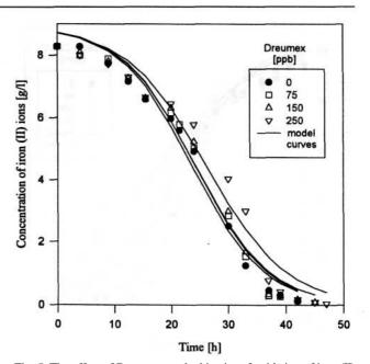
Fig. 5. The effect of Dreumex on the kinetics of oxidation of iron (II) ions by *Thiobacillus ferrooxidans* bacteria (Silverman 9K medium,  $37^{\circ}$ C, pH = 2.20).
