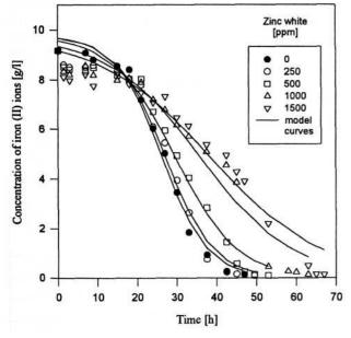
Fig. 1. The effect of zinc white on the kinetics of iron (II) ion oxidation by *Thiobacillus ferrooxidans* bacteria (Silverman 9K medium,  $37^{\circ}$ C, pH = 2.20).
